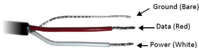
Figure 3: Pigtail End Wiring
