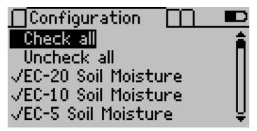
Navigate through the sensor list using' arrows. To change the status of a sensor, highlight it and press Enter. Each sensor name you check
