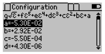
Each coefficient corresponds to a letter in the polynomial above. Below the polynomial resides the value of each coefficient in scientific notation. To edit a coefficient, press Enter while highlighting the coefficient. The Edit Screen appears to allow you to edit the coefficient.
