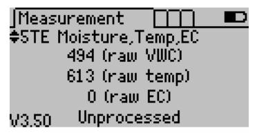
To modify the sensor calibration type, press Enter. You can choose a preset soil calibration type or create your own (See creating a Custom Calibration). To change the soil calibration type, select the medium option and press Enter. You can view the calibration coefficients by pressing Enter when the coefficients option is highlighted.
