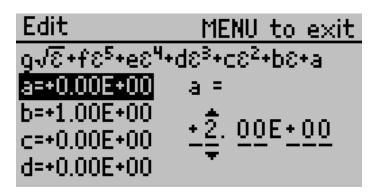
Use the arrow keys to change the current value, use the left and right arrow keys to change the cursor position.
