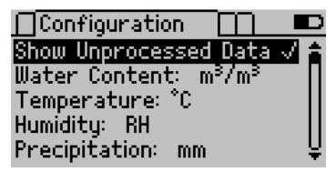
Use the arrows to navigate to the correct unit and press Enter to cycle through the unit options.
